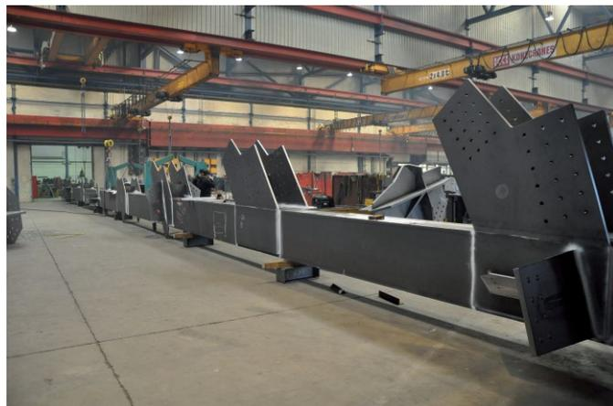
Fig. 11. Preassembly of the 40 m long truss chord for waste bunker in fabrication shop (by Züblin Stahlbau)
