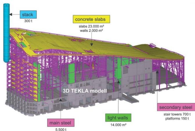
Fig. 3. 3D-TEKLA model – contract scopes of Züblin Stahlbau (by Züblin Stahlbau)
