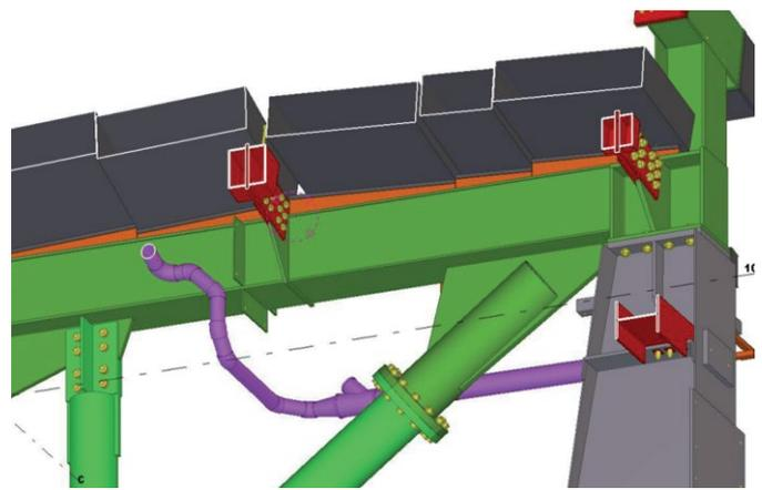
Fig. 6. 3D section through roof structure for process building (by Züblin Stahlbau)
