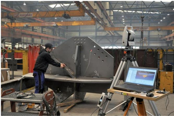
Fig. 9. 3D survey of column heads in fabrication shop (by Züblin Stahlbau)
