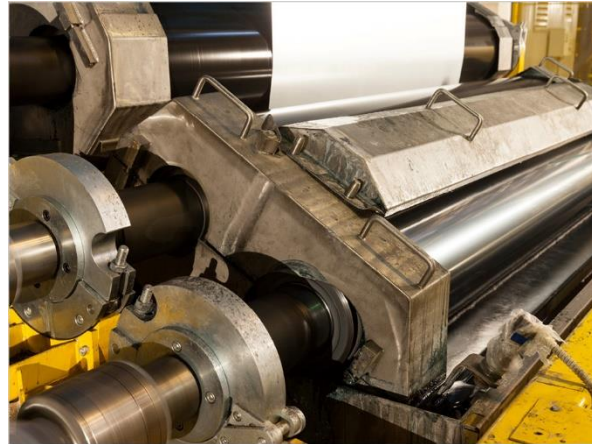
On-line application of thin organic coating
