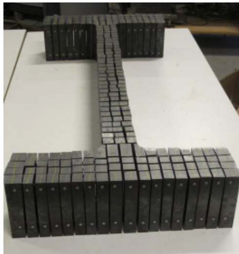
Complete sectioned specimen (HL920x1377)
