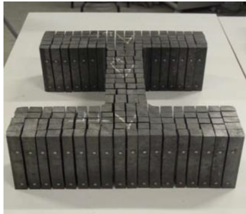
Complete sectioned specimen (HD400x1202)
