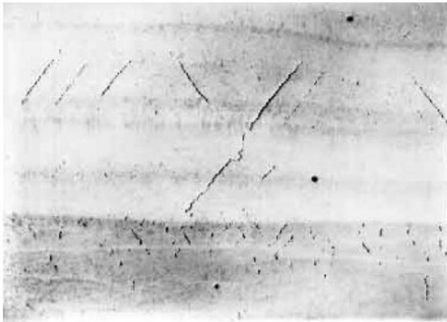
Longitudinal weld metal section showing 45° transverse or 'chevron' cracking
