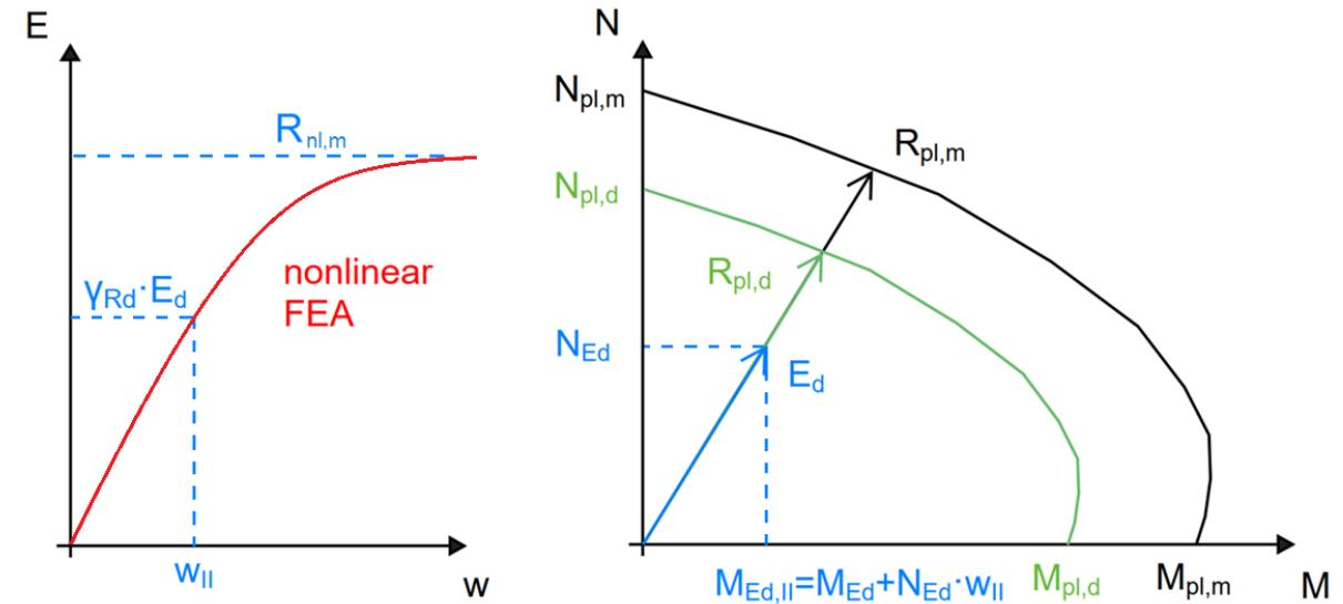
$$\gamma_{Rd} E (\gamma_g G_k + \gamma_q Q_k) \leq R \left( \frac{R_{nl,m}}{\gamma_0} \right) \quad \gamma_0 = \frac{R_{pl,m}}{R_{pl,d}}$$
