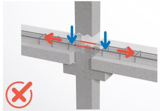
Inconvenient anchoring to reinforced concrete column
